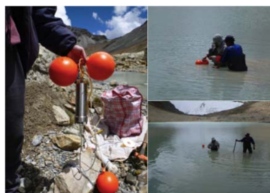
Turbidimeter installation in Huayna Potosi
