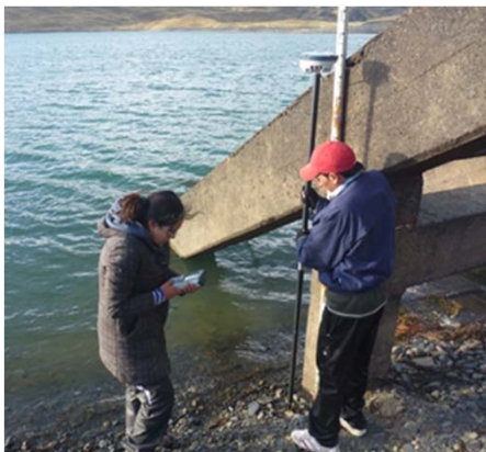
Photo: Measurement of sediment deposit in Tuni reservoir and 3D laser scanner
