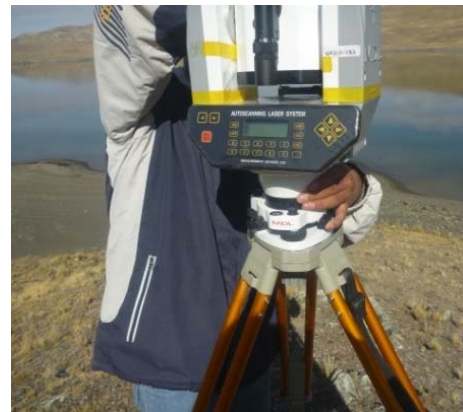
Photo: Measurement of sediment deposit in Tuni reservoir and 3D laser scanner
